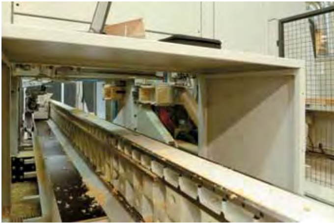
The Weinig Conturex enables manufacturers to produce wooden parts with any contours and of any batch size – in one through feed and with zero retooling time.
